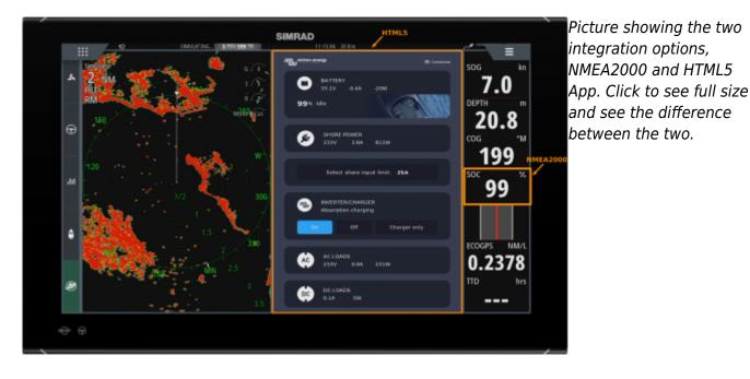
including Raymarine, Garmin, Navico and Furuno. Truly plug-and-play: once the Victron GX Device and the MFD are connected via ethernet, a Victron logo will appear in the App menu of the MFD. Behind that button, there is a page to monitor and control the Victron Energy system. The information on screen automatically adapts to the installed Victron system.
