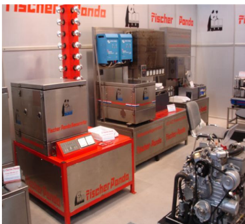
Phoenix Multi Plus on a Fisher Panda generator
